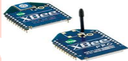
Figure 4: Zigbee module for wireless data communication
