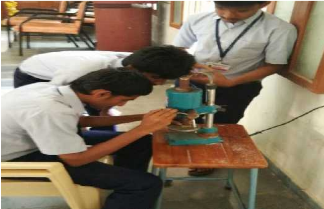
II ECE students using drilling machine to cut holes on the PCB
